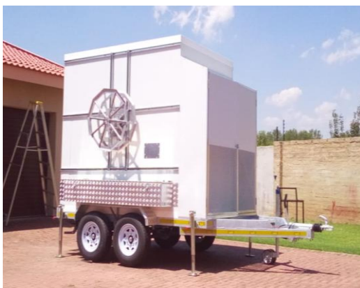
Figure 3: Trailer with sample line reel and data cable
