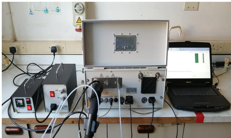
Figure 6: ProPAS – atmosFIR data acquisition system
