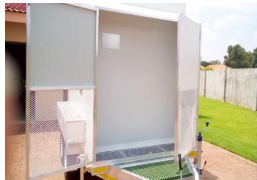
Figure 2: Trailer with aircon cage and gas cylinder cage
